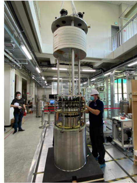
12 Tesla SC magnet 320mm bore diameter
